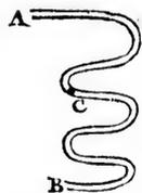
nel of brass, into which the ball C. is put, that runs down to B and falls into a frame, whence a ball is sprung up to the top of the frame, and falls into the channel at A.
