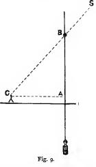
the angle at C to radius A C, or a rod with a scale of tangents drawn on it may be prepared from which the angle C will be directly read off.
