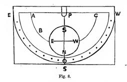
carrying a large-headed pin placed anywhere in the circle (s) in one of the sights. My first operation is to draw a correct meridian line (P s) on the clean deal surface. If the time is accurately known, this is at once performed by observing the shadow of the plumb line at the instant of true noon.
